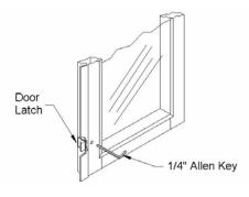
For units with a **GAL lock**, the door can be opened manually using a special key inserted into the round pin on the front of the lock (Figure 8).
